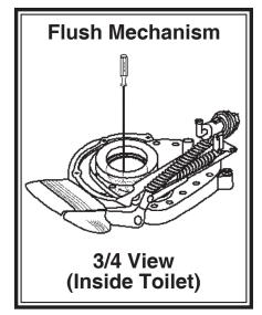
**Note**: Since cleaning of the seal groove is more pleasant after draining, rinsing and deodorizing the holding tank, we recommend that this be a routine procedure, rather than an on-the-road fix.
